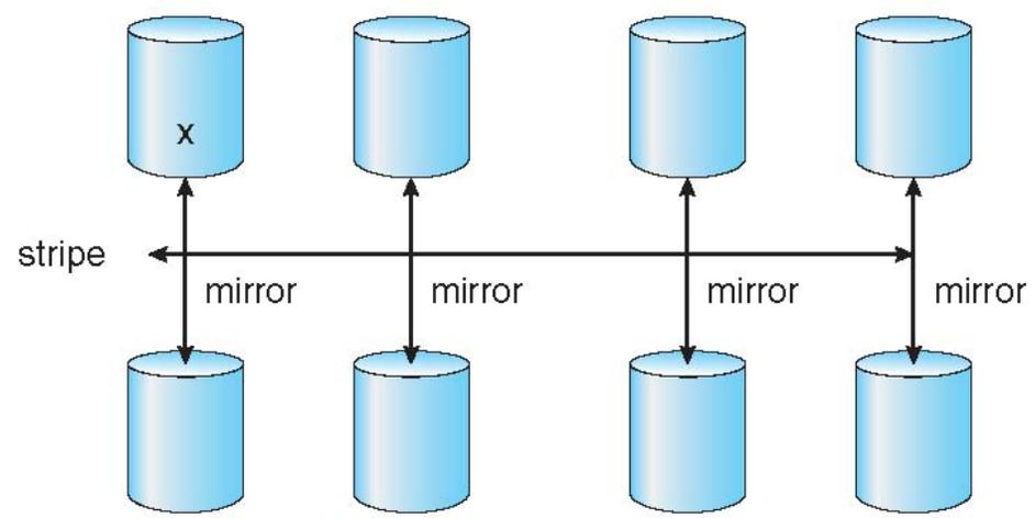
b) RAID 1 + 0 with a single disk failure.
